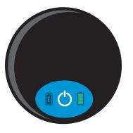
If the charger cannot find the generator within 90 seconds, it turns off automatically. If the charger turns off, press the power icon through the mesh pocket to turn the charger back on and realign it over your generator.
